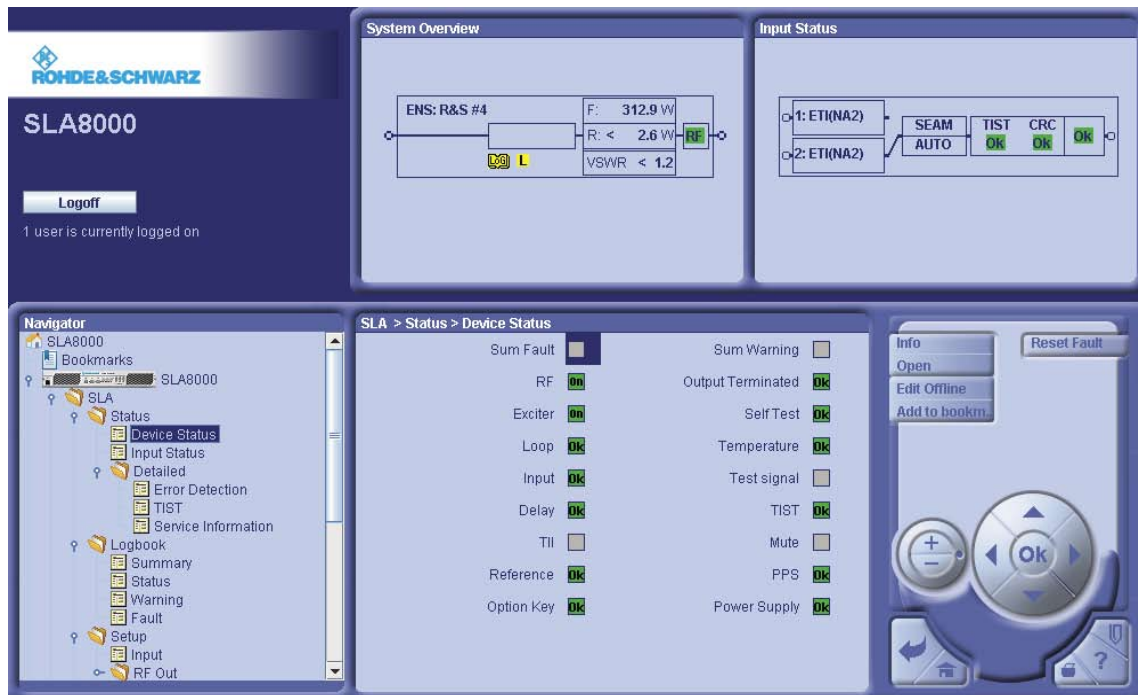
FIG 2 The transmitter status is displayed by the operating software of the R&S®SLA8000.
