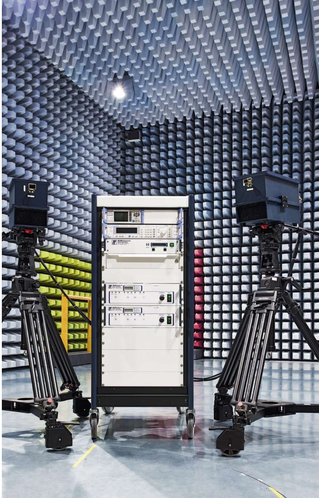
FIG 1 Amplifiers/antenna units detached from the preamplifiers generate field strengths of between 200 V/m and 300 V/m at a distance of 1 m at 40 GHz and with 40 W power.
