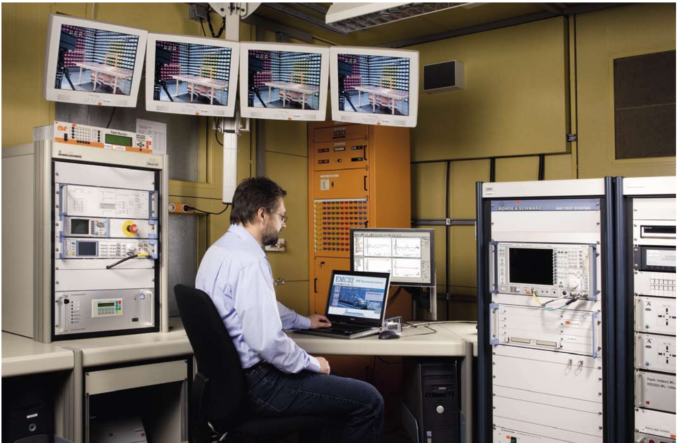
FIG 3 Each test chamber is permanently assigned a control room with test receiver, signal generator, power meter, EUT monitoring and measurement software from Rohde&Schwarz.
