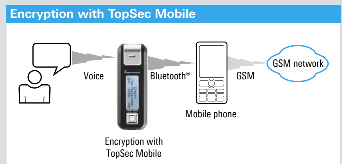
FIG 2 Mobile communications with the TopSec Mobile: The voice encryption device can be used with virtually all modern mobile phones.
