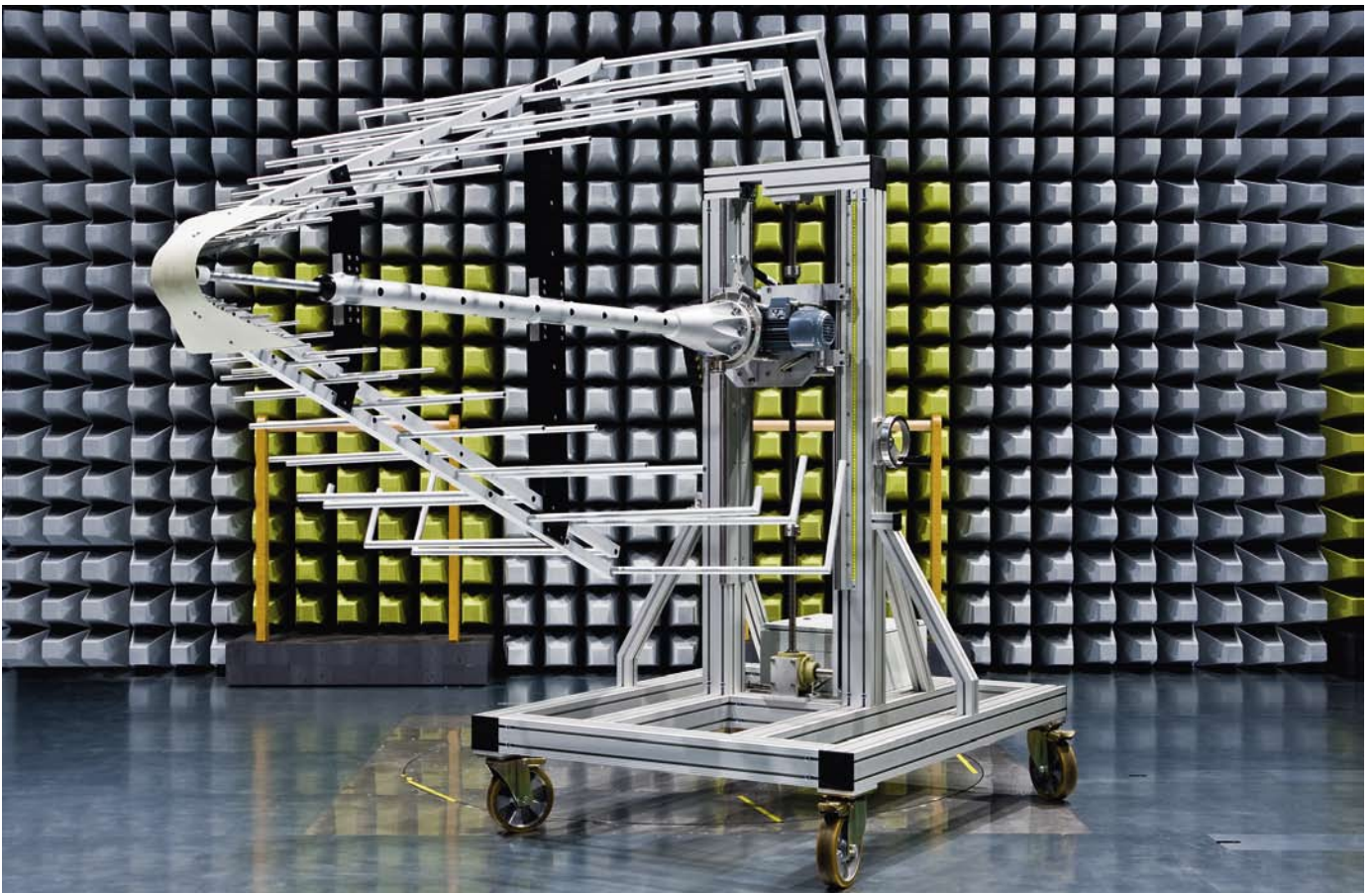
FIG 8 Above 80 MHz, compact directional LPD antennas are used to generate the required electromagnetic fields.
