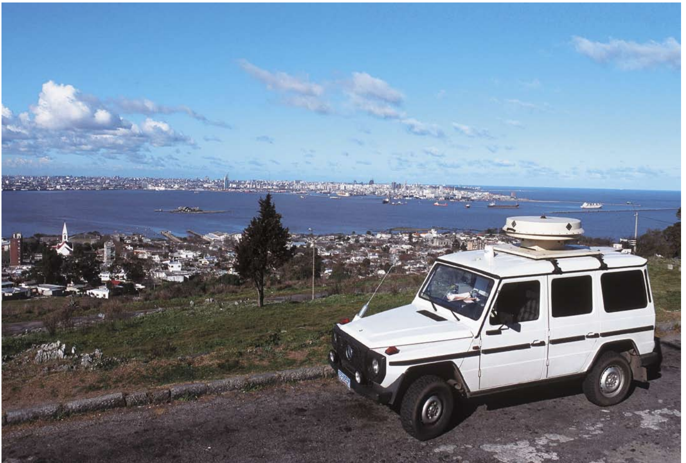
FIG 2 The R&S®ADD295 DF antenna mounted on the roof of an all-terrain vehicle.
